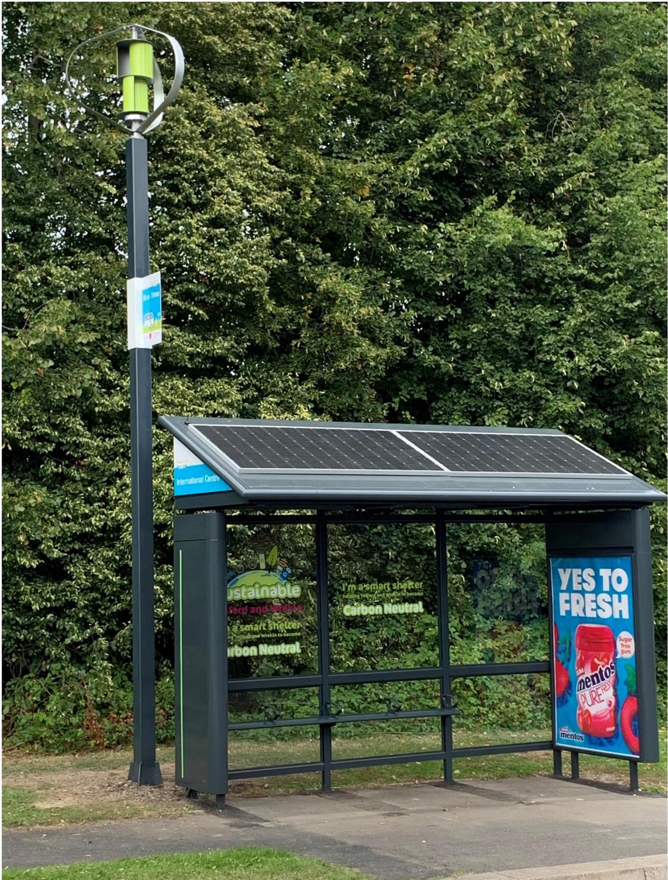
Figure 4-3 International Centre off-grid stop, with wind turbine and solar panels, e-ink display and QR code
